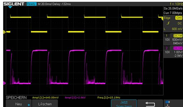
fig. 3 - Dots at a speed of 180 characters per minute.
