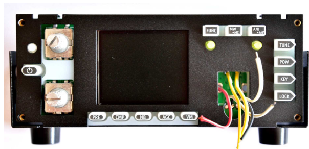
fig. 16 - Controller assembly fitted into the console.
