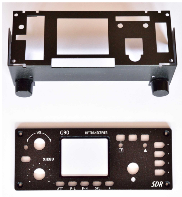
fig. 12 - Modified G90 console (top) and front plate (bottom).
